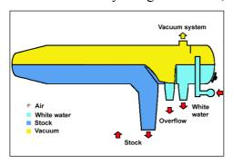
which may require chemicals or antifoam to work competently. However it is only functional with the help of a powerful vacuum pump which is an energy guzzler. The ultimate solution for de-foaming still depends heavily on the use of chemicals. Anti-foaming chemicals are pumped to the stock directly as an Add-on de-foaming
